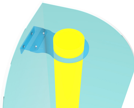
Step 3-4: After adjusting the brackets, secure the light column in place according to the desired length and height. The bracket holes may need to be drilled using a power drill to match the required height.
